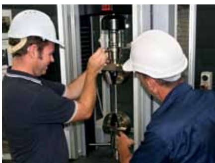
■ USC technical officers Bernhard Black and Hugh Allen set up for a tension and compression test.
